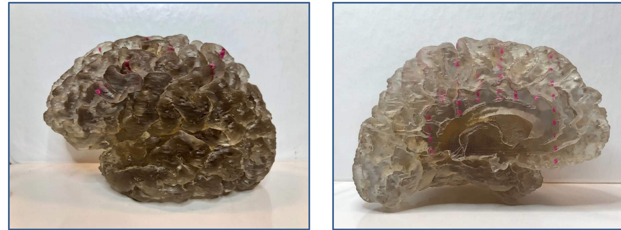
Figures 1 & 2. Rosary bead models generated from patient data printed on the Stratasys J750. Materials: VeroClear (brain mass) and VeroMagenta (electrode highlights).
