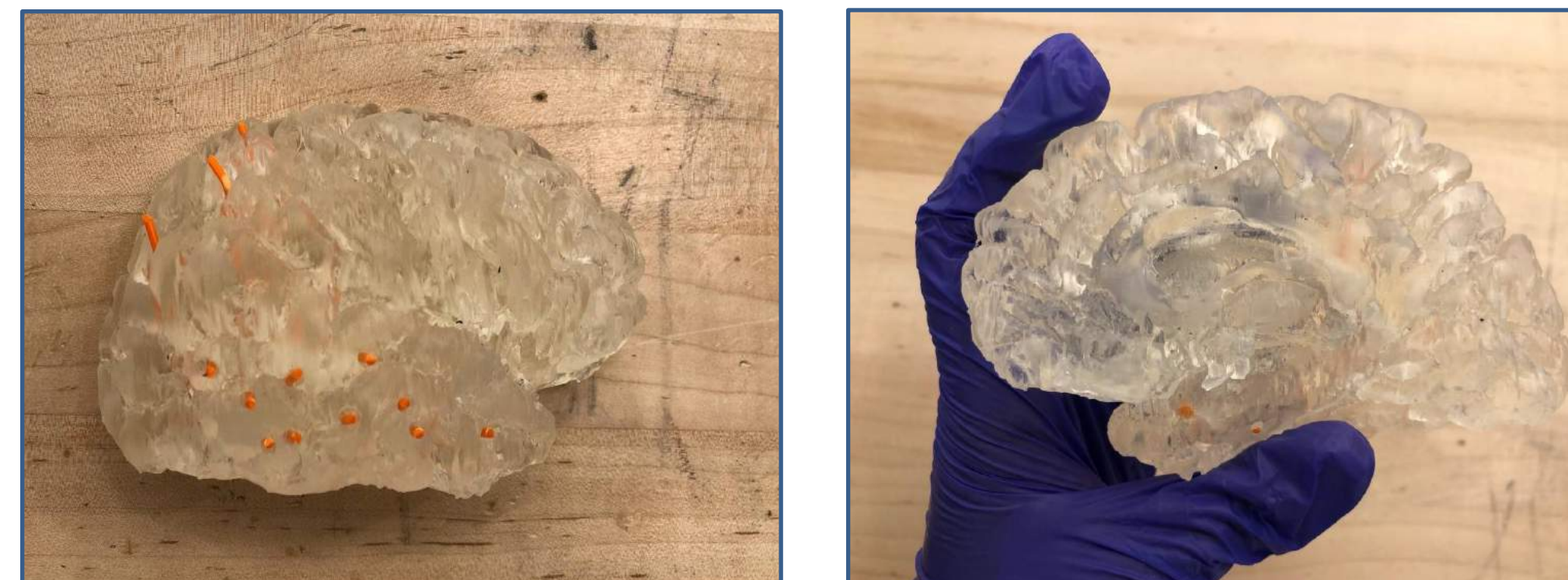
Figures 3 & 4. Swiss-Cheese models with inserted 'electrodes' printed on the Form 3. Brains were printed at 75% size due to buildplate limitations of the Form 3. Post-print UV curing was not performed to avoid cloudiness. Materials: SLA Clear
